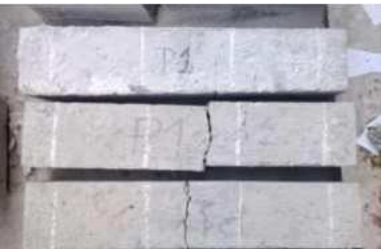
Fig. Failure of specimen under flexural tensile load
